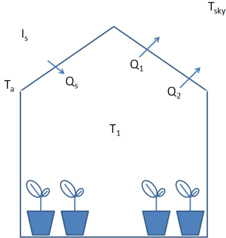
**Figure 1: Schematic diagram of the thermal transfer model for the farm greenhouse;**  $I_s$ , solar radiation;  $T_{sky}$ , sky temperature;  $T_1$ , internal temperature;  $T_a$ , ambient temperature;  $Q_s$ , solar energy;  $Q_1$ , energy flow to ambient atmosphere by heat transfer;  $Q_2$ , energy exchange by natural ventilation.
